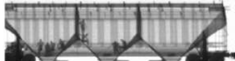
Fig. 3.1. "Railway wagon with illegal alien. The form of the wagon's loading spaces indicate design for coal or grain transport. Border Honduras, Mexico."
